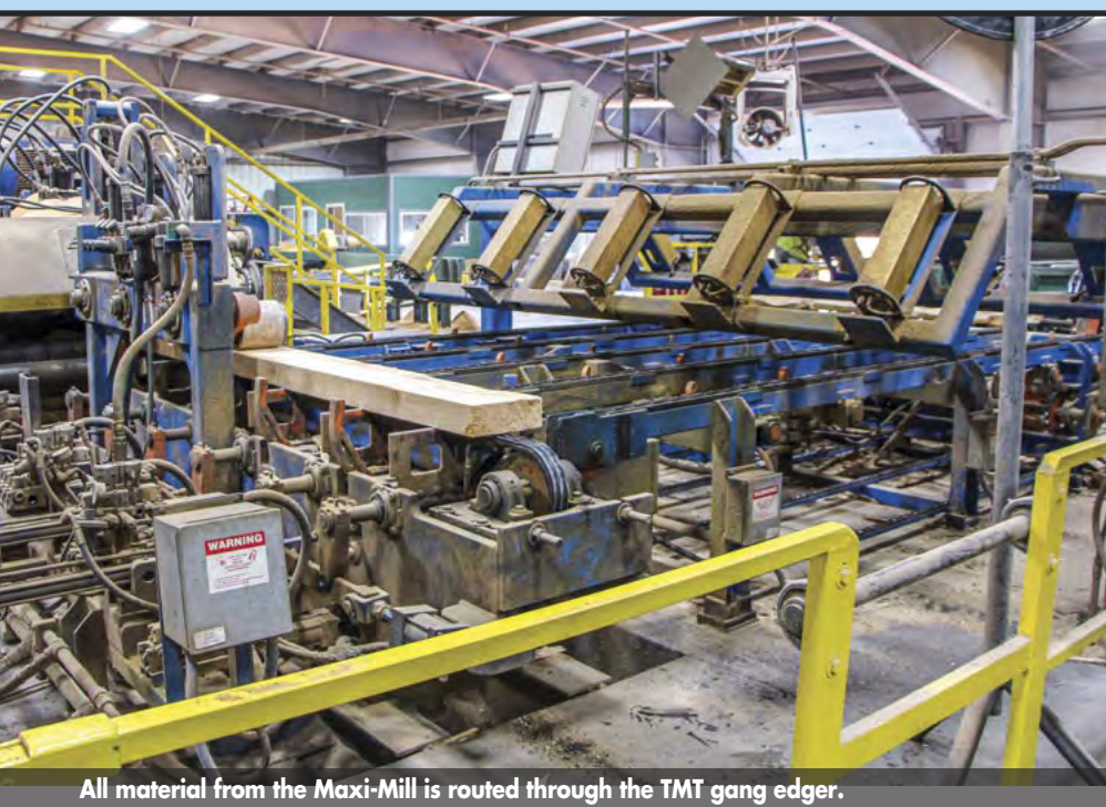
In this application, Maxi-Mill overhead end-dogging primary breakdown operates best as a single-pass machine.
